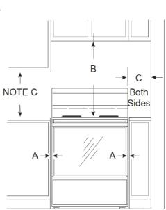
To reduce the risk of burns or fire when reaching over hot surface elements, cabinet storage space above the cooktop should be avoided. If cabinet storage space is to be provided above the cooktop, the risk can be reduced by installing a range hood that projects at least 5" beyond the front of the cabinets. Cabinets installed above the cooktop must be no deeper than 16".
