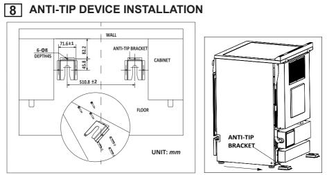
To prevent the range from tipping over due to improper use or overloading the open door, an antitip bracket (included in the package) must be installed properly by following instructions below. The anti-tip bracket can be fixed at either the left or right side of the appliance.
